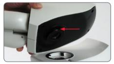
Install the eyepiece with the crossline reticle into the right eyetube so that the raised feature on the eyepiece aligns and is seated with the orientation slot in the right eyetube.
